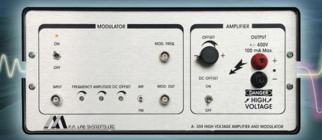
The A-304 piezo Driver/Piezo Amplifier is a high Voltage, high speed Piezo Driver / Linear Amplifier combined with a wide band AM/FM modulator.
